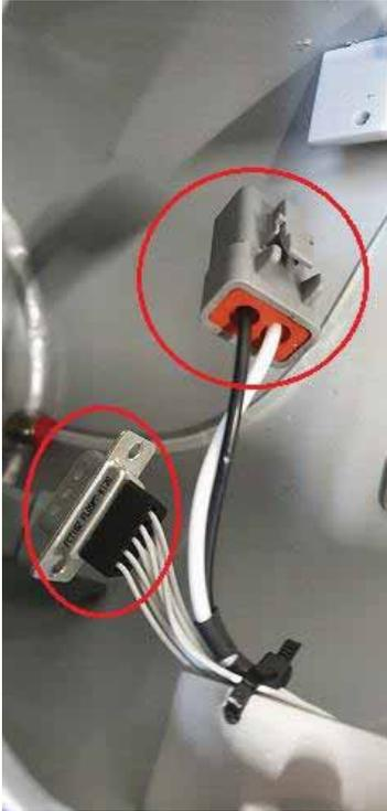
Figure 31 - Power and communication connectors
