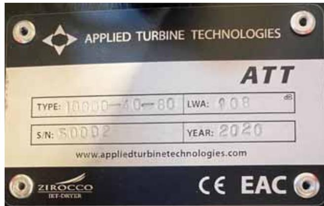
The Hammer Jet has an A-weighted max sound power level of 108 dBA around the machine and **103 dBA at the operators’ position**, at its max performance. The LWA is here not directly related to an environmental noise level as weighted average of the different work steps during machine operation. It is the maximum sound pressure which the operator will experience when using the machine at 100% performance level.
