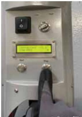
Figure 14 - Step 3: reset the ECU
