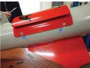
Figure 38 - Filter cover screws
