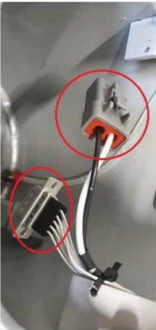
Figure 26 - Communication and power connector
