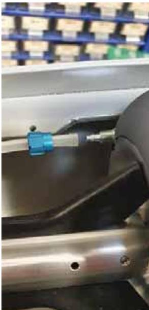
Figure 32 - Loose fuel connection
