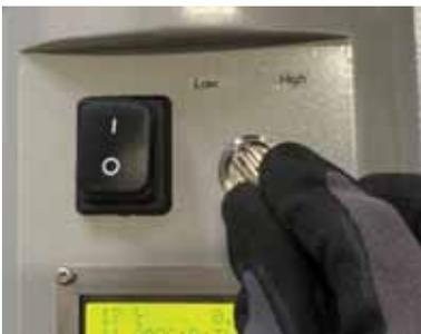
Figure 16 - Step 6: Option “Low” or “High” on the Power button
