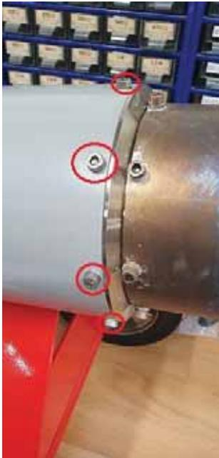
Figure 24a- Socket and head bolts
