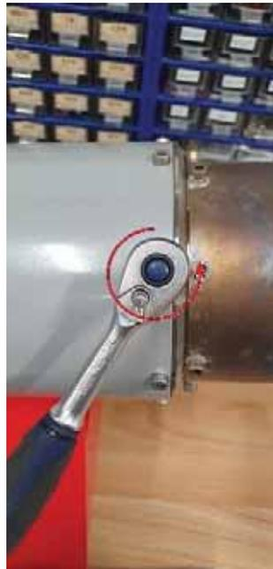
Figure 24b - Unscrewing the socket heads
