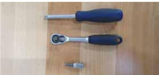
Figure 37 - Filter removal tools
