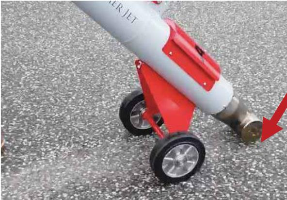
Figure 6 – Nozzle opening position for optimal drying speed.
