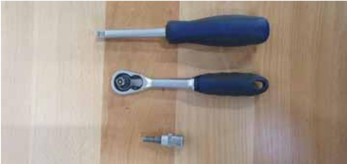
Figure 23 - Tools for dismantling the turbine module
