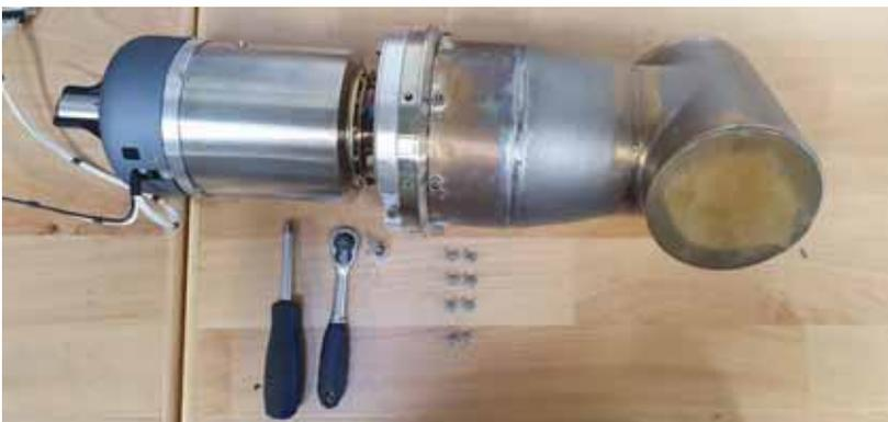
Figure 28 - Turbine module installation tools
