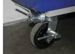
Rear Wheel System with release and brake.
