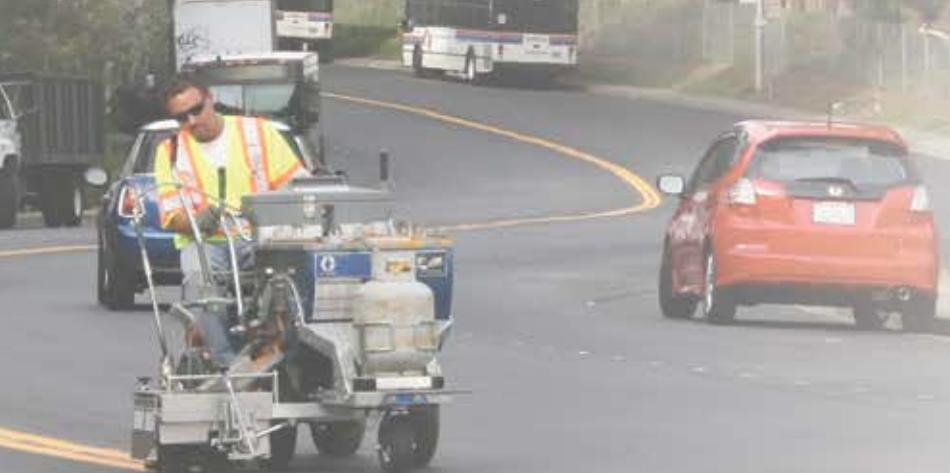
**LineDriver System** Get higher productivity with less fatigue by riding instead of walking with the patented LineDriver and LineDriver HD Systems.
